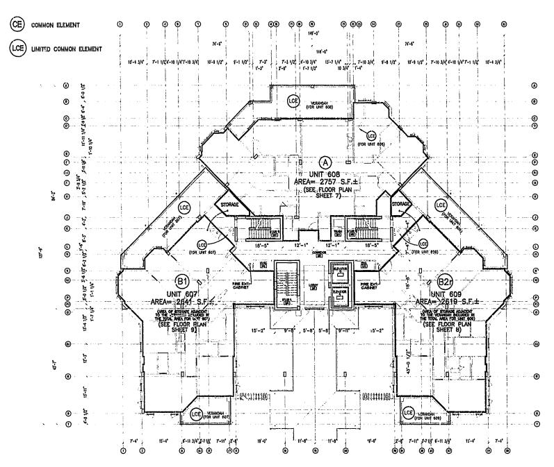
NOTE: BOLD DIMENSIONS ARE BASED UPON ACTUAL FIELD MEASUREMENTS TAKEN AT OUTSIDE FACE OF BRICK. OTHER BUILDING DIMENSIONS AND DETAILS SHOWN ARE PER PLANS BY NCG ARCHITECTS INCORPORATED.
