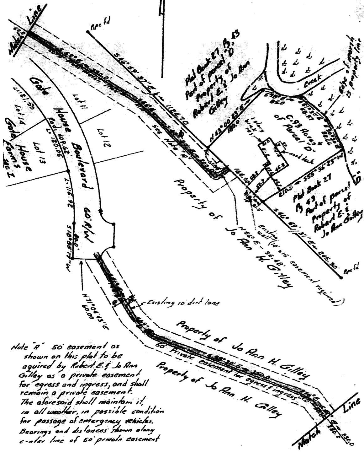
Note "A" 50' easement as shown on this plot to be acquired by Robert E. & Jo Ann Gilley as a private easement for egress and ingress, and shall remain a private easement. The aforesaid shall maintain it, in all weather, in possible condition for passage of emergency vehicles. Bearings and distances shown along center line of 50' private easement
