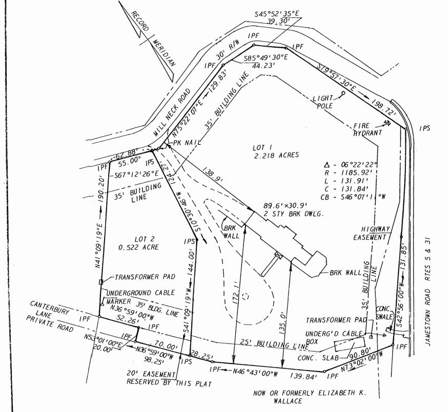
VEHICULAR ACCESS TO LOT 2 IS LIMITED TO CANTERBURY LANE OR BY THE EXISTING RIGHT OF WAY OVER LOT I TO MILL NECK ROAD. ALL UTILITIES ARE TO BE INSTALLED UNDERGROUND.
