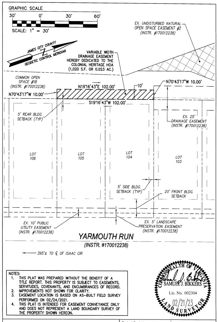
PLAT SHOWING VARIABLE WIDTH DRAINAGE EASEMENT LOCATED ON COMMON OPEN SPACE #1B WITHIN COLONIAL HERITAGE PHASE VI, SECTION 1B
