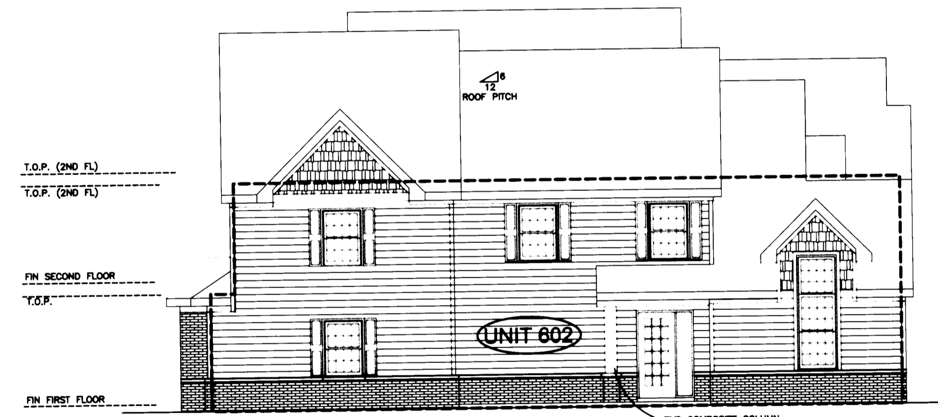
RIGHT SIDE ELEVATION- MODEL B (UNIT 602) 1/8" = 1'-0"
