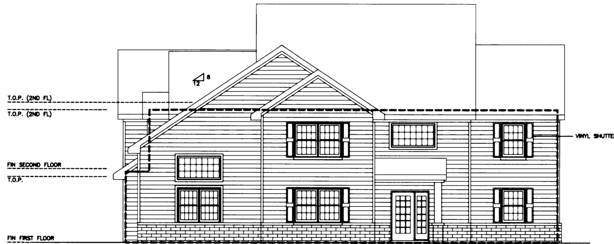
LEFT SIDE ELEVATION- MODEL A (UNIT 101) 1/8" = 1'-0"
