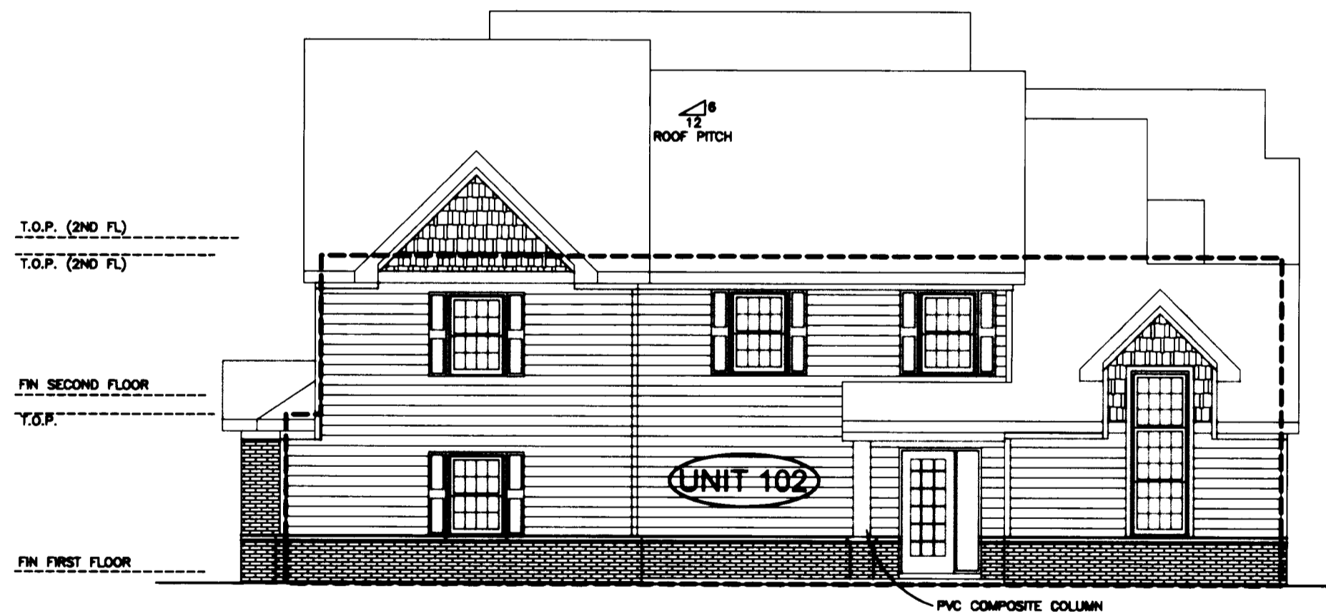
RIGHT SIDE ELEVATION- MODEL B (UNIT 102) 1/8" = 1'-0"
