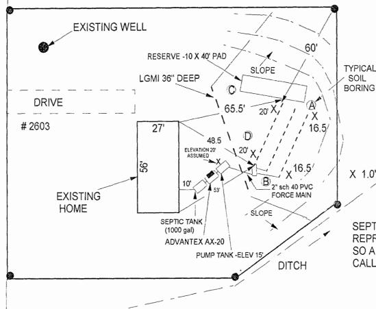
INSTALL 3-43.75' DRAINLINES INSTALL TRENCH BOTTOM - 116" USE INFILTRATOR TRENCH SECTIONS ON 9'CENTERS WITH 3' WIDE TRENCH GRADE SURFACE TO DRAIN
