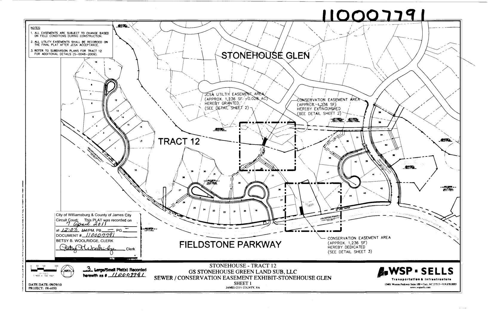
197791 NOTES: 1. ALL EASEMENTS ARE SUBJECT TO CHANGE BASED ON FIELD CONDITIONS DURING CONSTRUCTION. 2. ALL UTILITY EASEMENTS SHALL BE RECORDED ON THE FINAL PLAT AFTER JCSA ACCEPTANCE. 3. REFER TO SUBDIVISION PLANS FOR TRACT 12 FOR ADDITIONAL DETAILS (S-0048-2009). JCSA UTILITY EASEMENT AREA (APPROX. 1,236 SF -0.028 AC) HEREBY GRANTED -CONSERVATION EASEMENT AREA (APPROX. 1,236 SF) HEREBY EXTINGUISHED 34 STONEHOUSE - TRACT 12 M-WSP - SELLS GS STONEHOUSE GREEN LAND SUB, LLC
